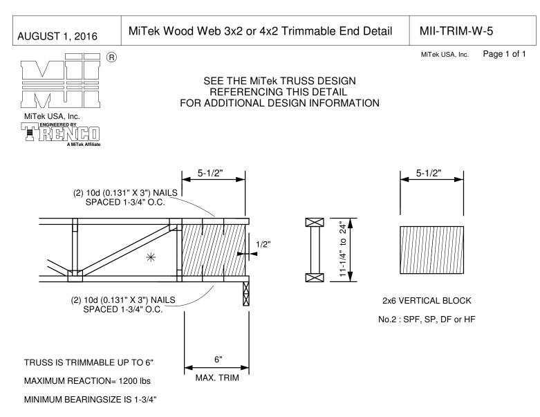
st last diagonal web must be ran up to the top chord as shown
