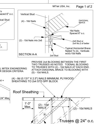
Typical \_x4 L-Brace Nailed To Verticals W/10d Nails spaced 6" o.c. Vertical Stud SECTION B-B DIAGONAL BRACE TRUSS GEOMETRY AND CONDITIONS 4'-0" O.C. MAX SHOWN ARE FOR ILLUSTRATION ONLY. Varies to Common Truss SEE INDIVIDUAL MITEK ENGINEERING DRAWINGS FOR DESIGN CRITERIA \*\* 3x4 =
