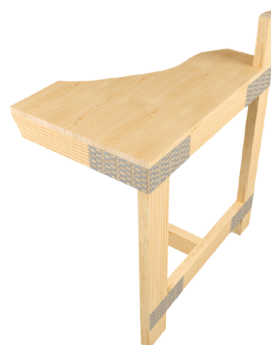
Typical mending plate installation
