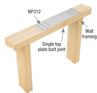
Typical NP312 prescriptive top plate splice installation
