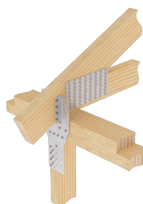
Typical LUGT1 offset stud installation (See footnote #4)
