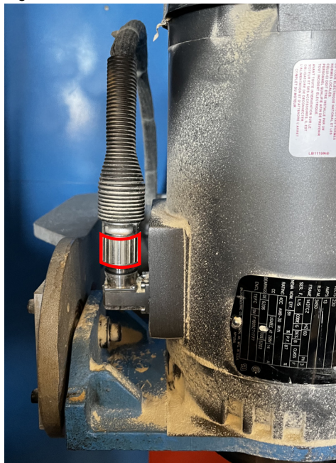
Figure 5: Disconnect Power Cable
