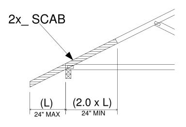
NOTE: TRUSS BUILT WITHOUT AN OVERHANG. THIS DETAIL IS NOT TO BE USED WHEN OVERHANG HAS BEEN BROKEN OFF.
