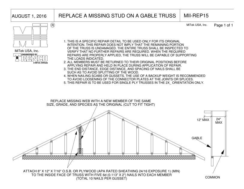
THE OUTSIDE FACE OF THE GABLE MUST BE SHEATHED WITH (MIN) 7/16" O.S.B OR PLYWOOD. SEE MITEK STANDARD GABLE END DETAILS FOR WIND BRACING REQUIREMENTS.
