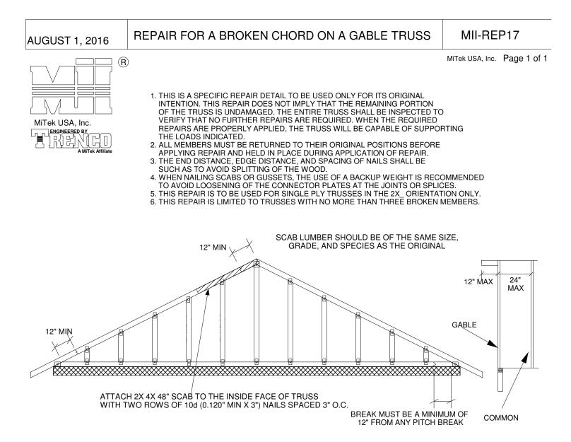
THE OUTSIDE FACE OF THE GABLE MUST BE SHEATHED W/ (MIN) 7/16" O.S.B OR PLYWOOD. SEE MITEK STANDARD GABLE END DETAILS FOR WIND BRACING REQUIREMENTS.
