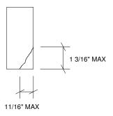
SPLIT MUST NOT EXTEND UNDER CONNECTOR PLATE
