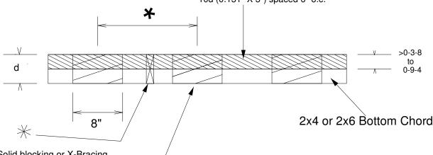
Solid blocking or X-Bracing spaced 48" on center required when padding up the bottom chord greater than 0-7-4 past it's original height.
