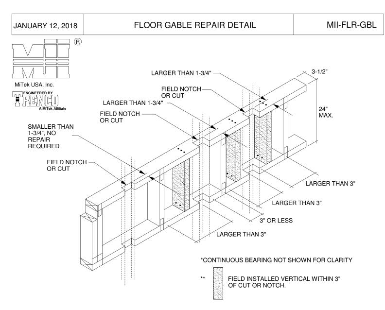
FLOOR GABLES(S) (LADDER TRUSSES) ARE CONVENTIONAL WALLS WITH CONNECTOR PLATES PER ANSI/TPI1 SECTION 6.6 AND USED IN CONVENTIONAL WALL FRAMING MEETING IRC SECTION R602. REFER TO MITEK/TRENCO DESIGN DRAWING FOR MATERIAL SPECIFICATIONS.
