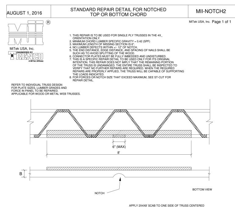
APPLY 2X4X8' SCAB TO ONE SIDE OF TRUSS CENTERED ON NOTCH WITH CONSTRUCTION QUALITY ADHESIVE AND 1 ROW OF 10d (0.131" X 3") NAILS SPACED 3" O.C. SCAB GRADE AND SPECIES TO MATCH EXISTING CHORD.
