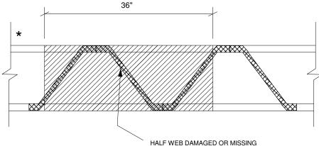
ATTACH 3/4" PLYWOOD OR OSB GUSSET (23/32" APA RATED SHEATHING 48/24 EXP 1) TO EACH SIDE OF TRUSS WITH CONSTRUCTION QUALITY ADHESIVE AND ONE ROW OF 10d (0.131" X 3") NAILS SPACED 3" O.C. FROM EACH FACE.
