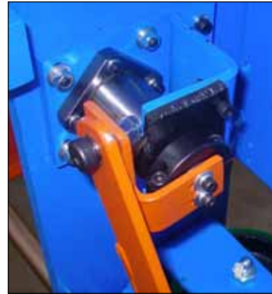
Figure 6: Attach Dog-Leg Assembly to Bumper Shaft
