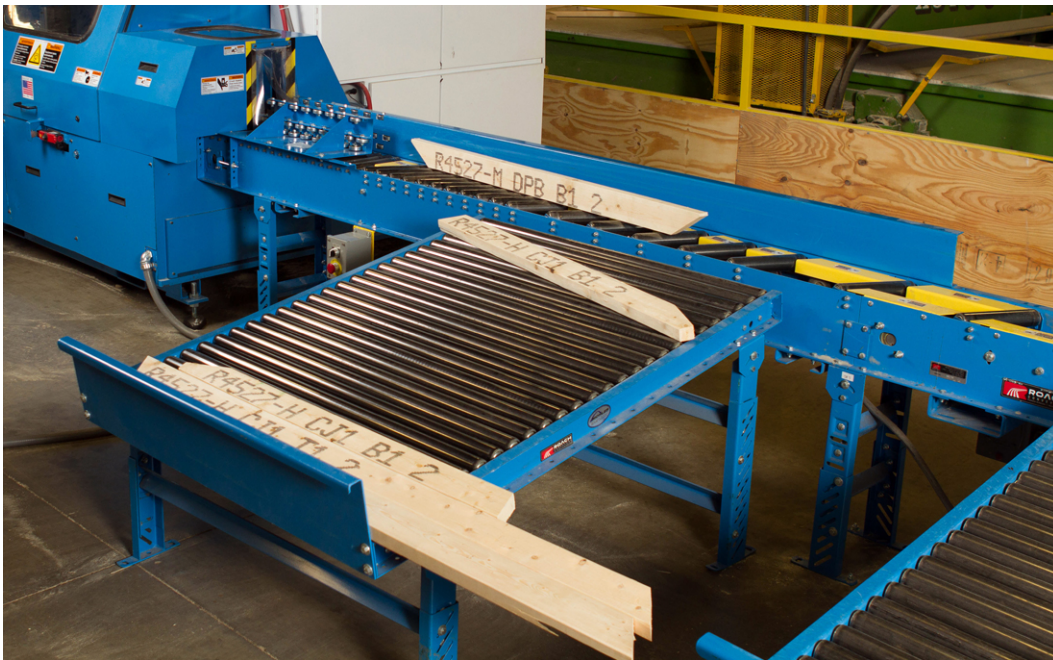
Figure 2-4: Optional Powered Skewed Conveyor Attached to Saw
