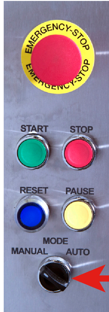
Figure 4-30: Mode Selector Switch Shown in Manual Mode
