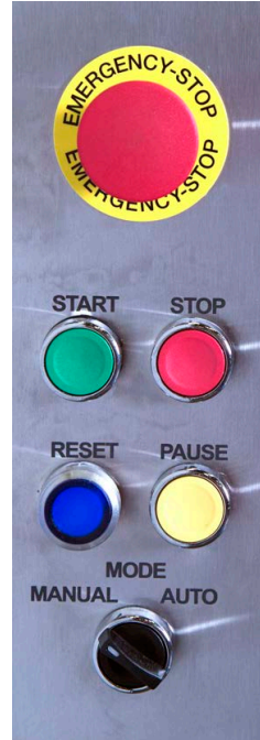
Figure 4-16: Mechanical Controls on Operator Interface Panel
