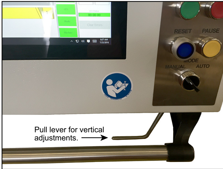
Figure 4-15: Moving the Touch Screen Up and Down
