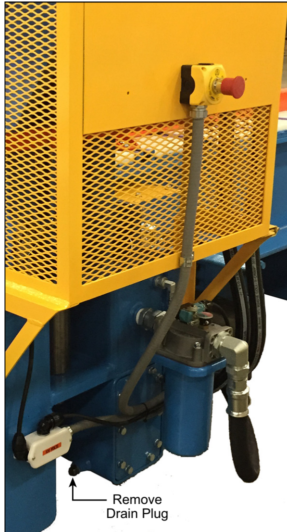
Figure 7-6: Draining the Reservoir
