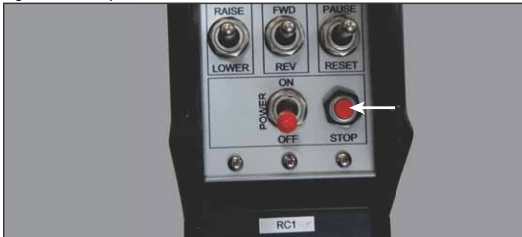
Figure 5-3: E-Stop Pushbutton on Radio Controller
