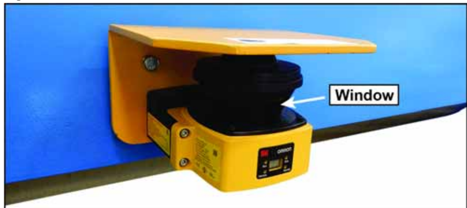
Figure 7: Laser Scanner Window Location
