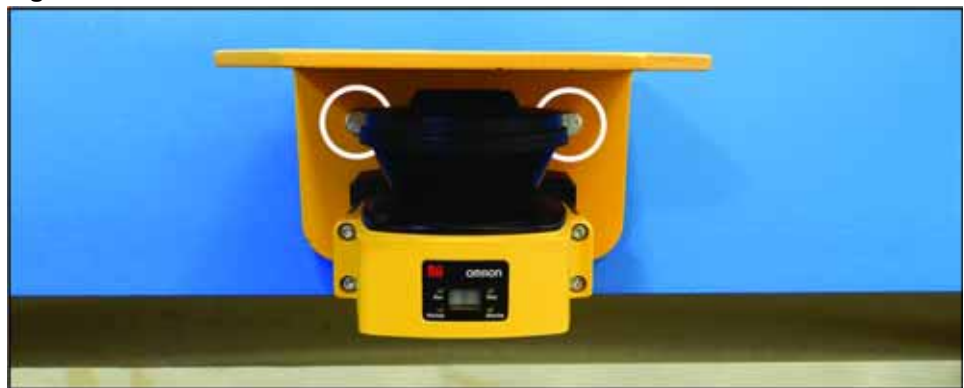
Figure 4: Screw Locations on Laser Scanner Mount
