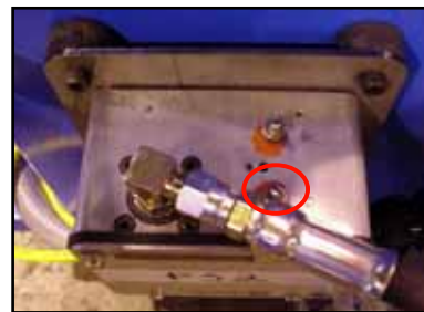
Figure 3-15: Pressure Switch Adjustment
