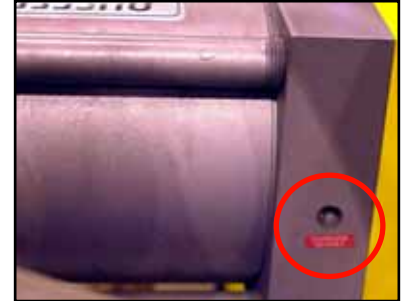
Figure 3-16: Cushion Adjustment Screw
