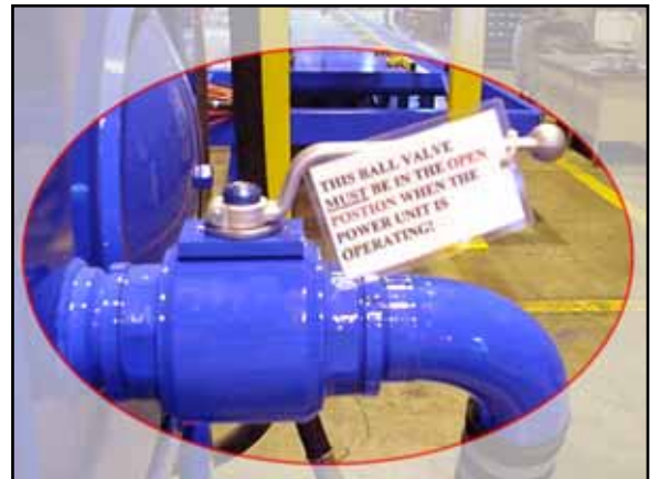
Figure 3-9: Suction Line Ball Valve
