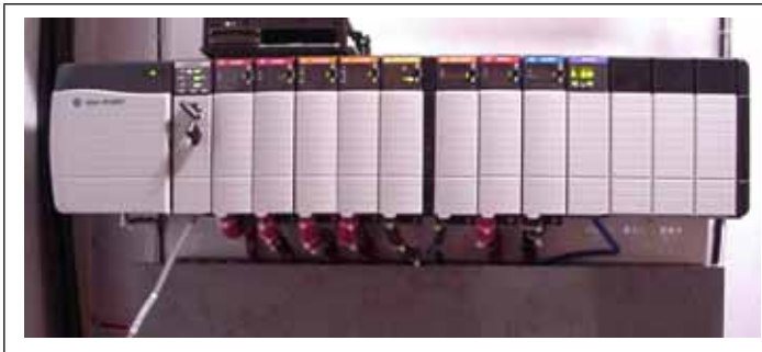
Figure 3-25: PLC Controller and Input/Output Cards
