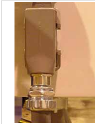
Figure 3-21: Port on Press Junction Box
