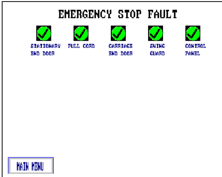
Figure 6-8: Emergency Stop (E-Stop) Fault Screen
