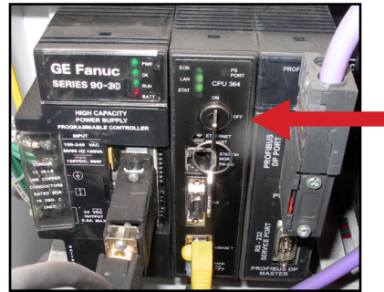
Figure 7-37: Turn Key TWICE to Reset the PLC
