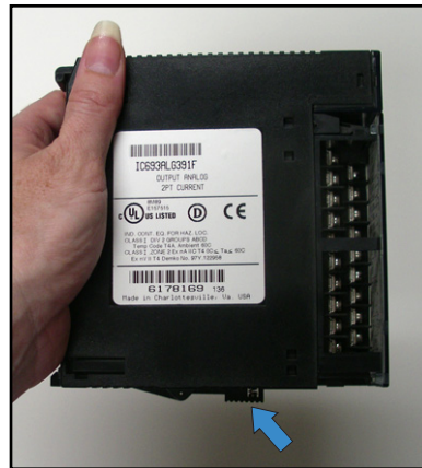
Figure 7-39: Press Release Latch to Remove Card
