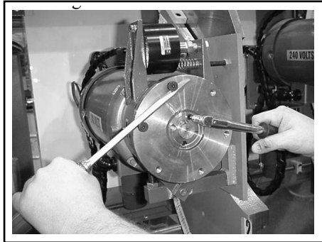
Figure 6-14: Tighten Hub Screws
