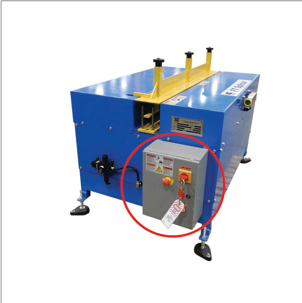
Figure SAFETY-1: Lockout/Tagout on the Main Electrical Enclosure
