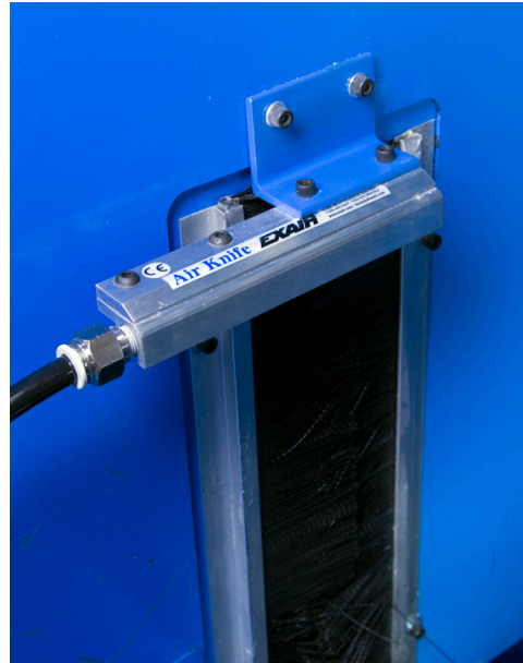
Figure 2-61: Air Knife Inside Saw Chamber
