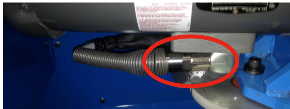
Figure 2-97: Connection Point at Saw Blade Motor
