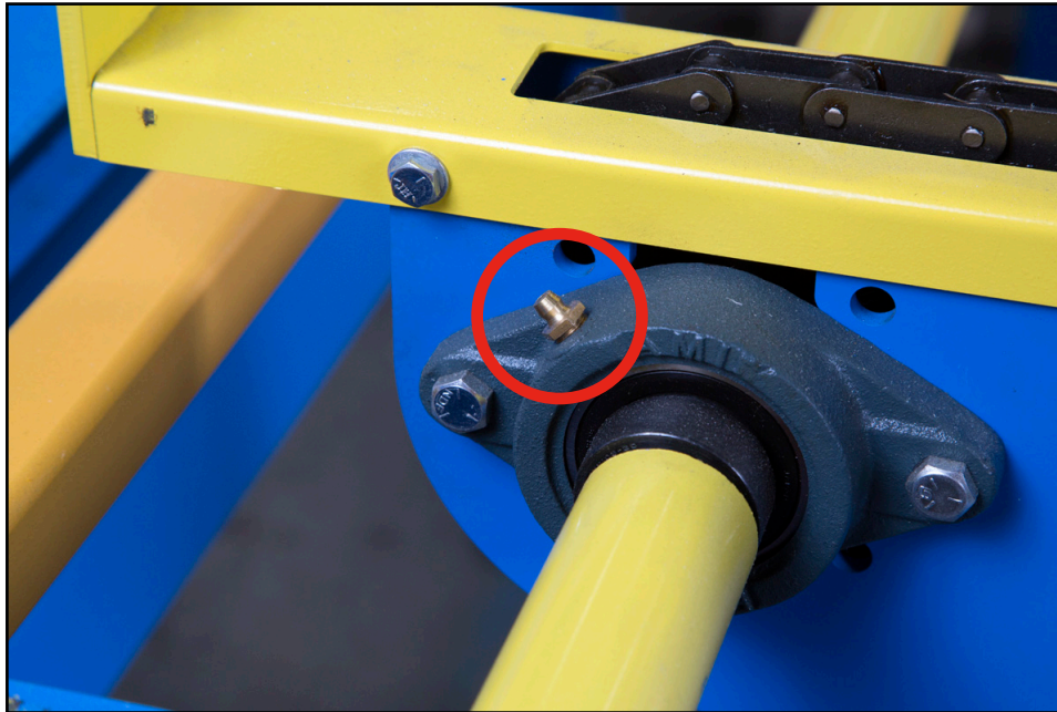
Figure 2-21: Grease Fitting for Auto Deck Shaft
