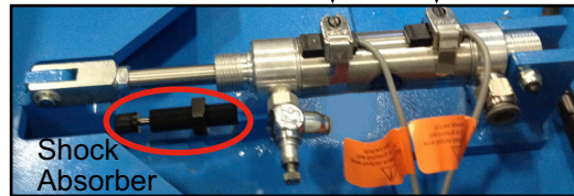
Figure 2-39: Outfeed Clamp Adjustment
