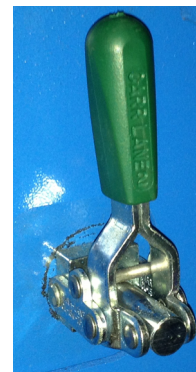
Figure 2-28: Raising the Infeed Clamp & Printer Assembly
