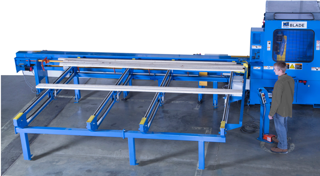
Figure 2-3: Auto Deck as Part of a MatchPoint BLADE Wood Processing System
