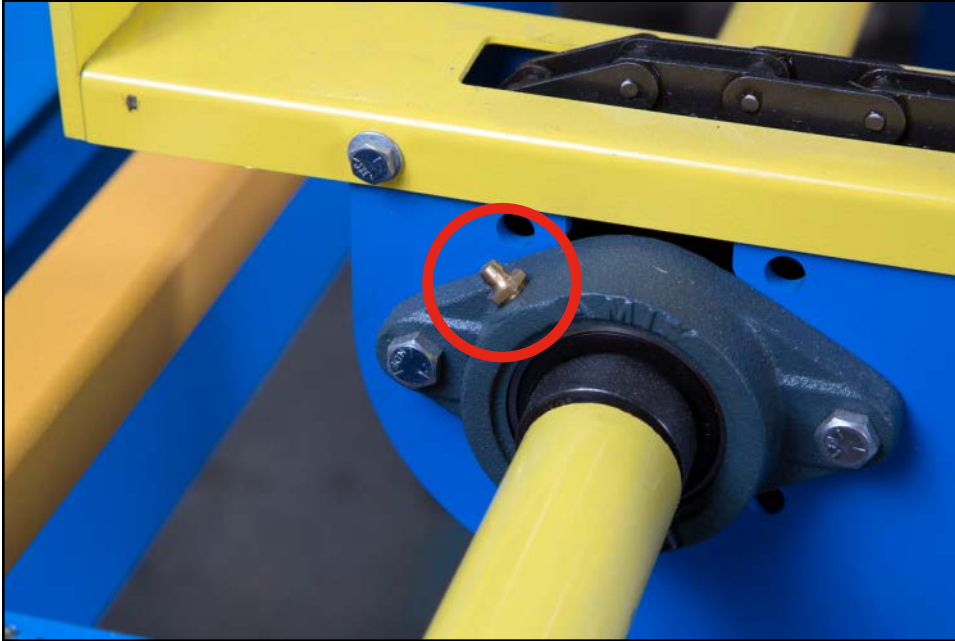
Figure 7-40: Auto Deck Drive Shaft Grease Fitting Location
