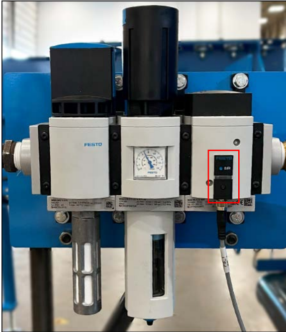
Figure 7-65: Pressure Sensor Adjustment on Main Filter/Regulator Assembly
