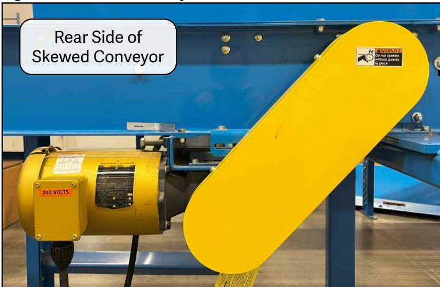
Figure 7-43: Skewed Conveyor Chain Lubrication Point
