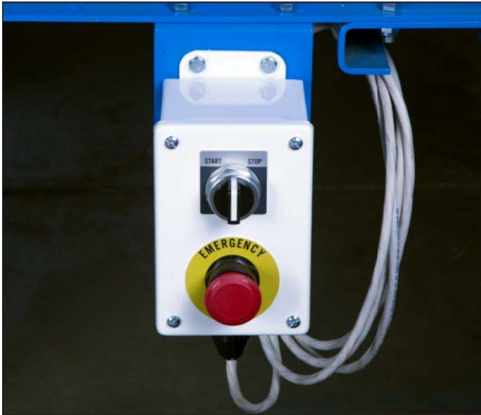
Figure 6-9: Skewed Conveyor Controls
