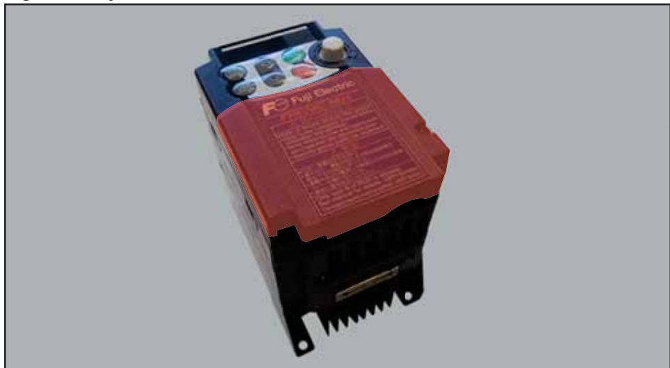
Figure 2: Fuji VFD Control Circuit Terminal Block Cover
