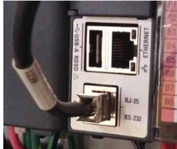
Figure 16: Connect the Touchscreen Cable
