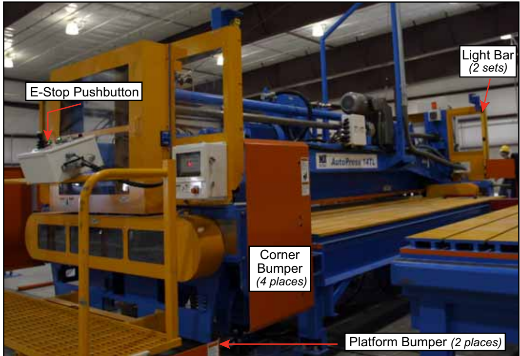
Figure 6-1: How to Stop the Gantry Head
