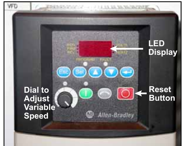
Figure 7-19: Controls on the VFD
