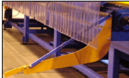
Figure 3-10: Outfeed Arm Assemblies
