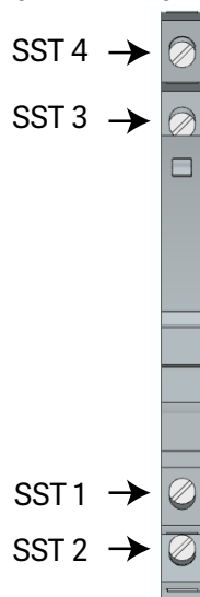
Figure 11: Surge Suppressor Terminal Locations
